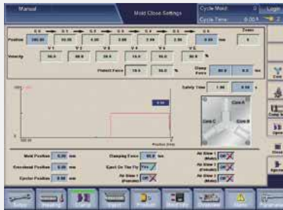
Mold protection function with 2 steps in standard.
