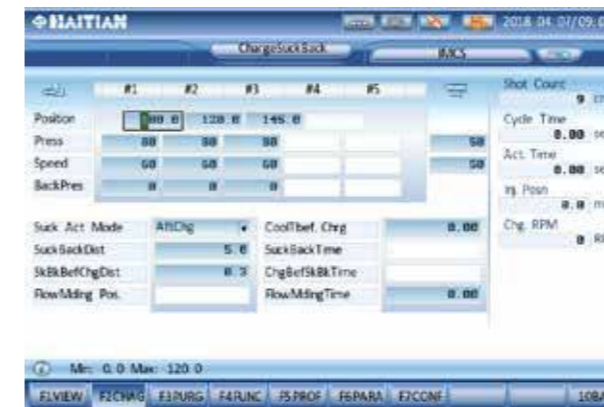
Charge screen: Back pressure proportional valve control
