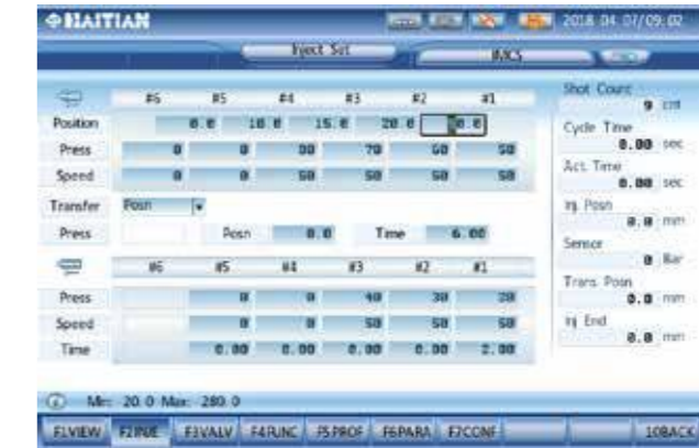
Injection screen: 6 stage injection control
