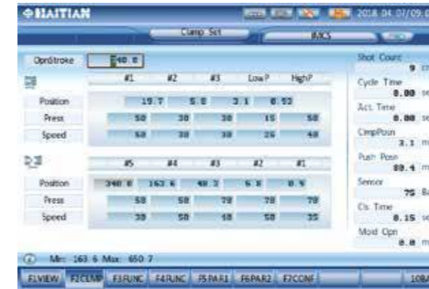
Mold screen: Mold opening/closing position precise control
