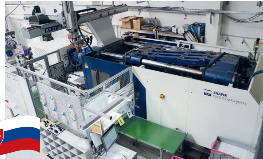
In a direct comparison test between a VE 4500 II and a corresponding hydraulic machine, Venus II reached a value of energy below that of 75 % of the competitive machines.
