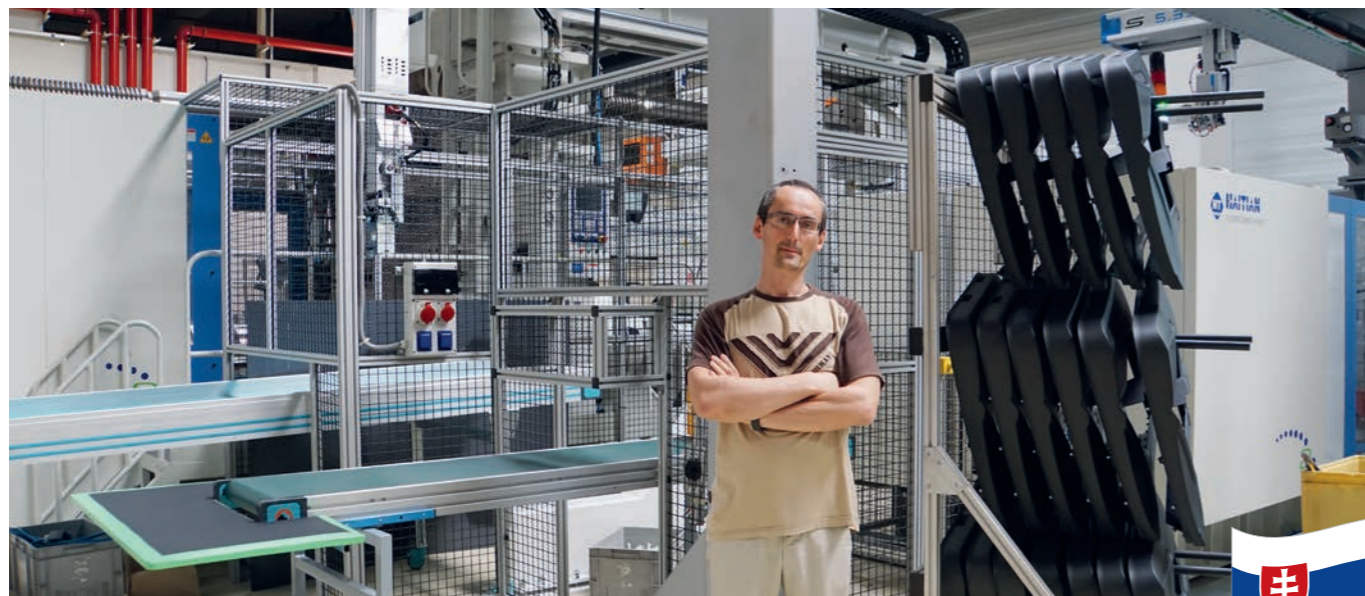
Behind Milan Večera stays a JU 24000 II, producing door trims for VW Caddy.
