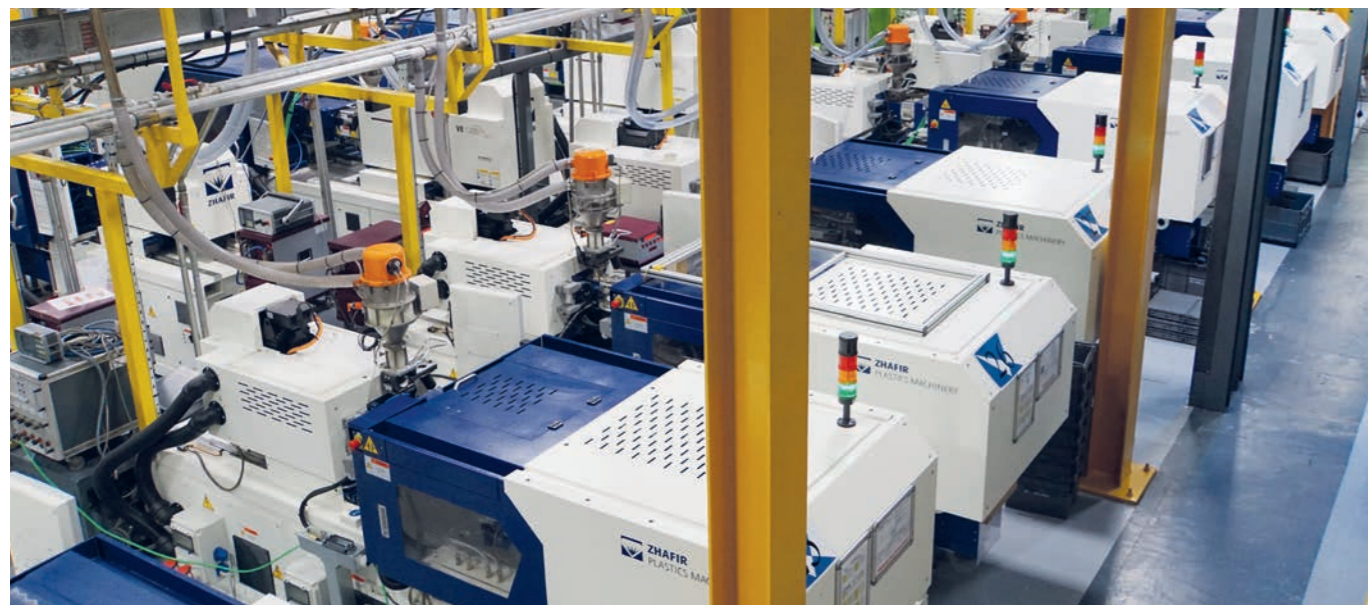
17 electrical injection molding machines bear the logo of the Venus II Series, working with clamping forces of between 600 and 1,200 kN.
