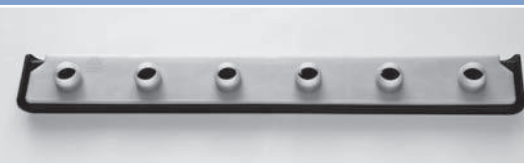
Lower part (black) made from PP regranulate, part weight 58.3 g + 1.5 g sprue, and cover, (white) made from PP+TPE, part weight 26.3 g + 1.5 g sprue; both produced in 4 cavities, with a cycle of between 24 and 30 seconds
