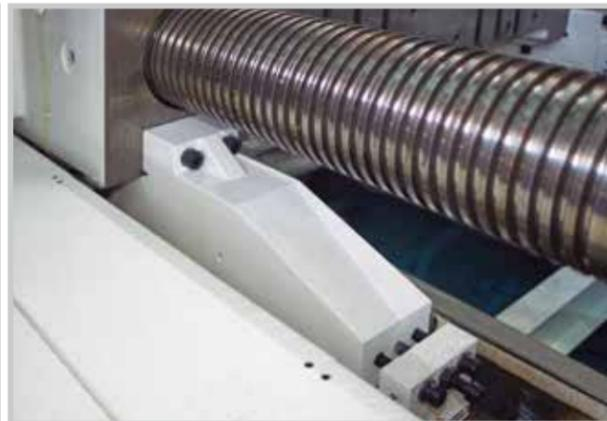
The compact design of the two-platen clamping structure has been integrated into the JE series, with optimized space layout and providing larger mold space, extended mold movement stroke and ejector stroke.
